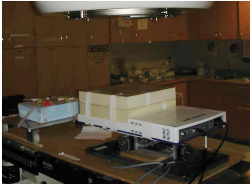
**Figure 3.** Experimental setup for the dosimetric study: a commercial diode array was placed on the top platform of the motion phantom and covered with water-equivalent material with a total thickness of 10 cm. The linac gantry was at  $0^\circ$ .
